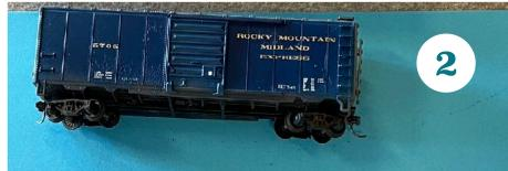
This boxcar was airbrushed at last month's clinic. (for passenger service) Notice the waybill "copies" tacked to the "boards" on the doors and car ends. Notice the patterns of "wheel grime" on the car ends.
