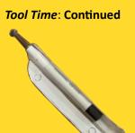
Nick Muff showed a small, retractable steel bristle brush, which is good for scratching paint to suggest peeling paint (on a structure), as well as cleaning wheel treads and myriad other uses. This usually comes as a set of 4 brushes, also including brushes with brass and fiberglass bristles.
