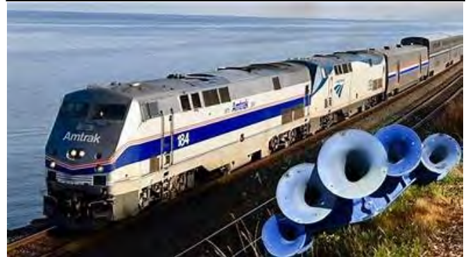
This Nathan K5LA five-chime assembly has five "bells" whose musical chord helps the horn to be heard and lessens complaints. The bells may be reversed for trains that go backwards and help those working at the back of the train hear the horn on the front. The K5LA is the most popular horn in use today. For those musically inclined it has a B major 6th chord (D-sharp, F-sharp, G-sharp, B, D-sharp). Though first used by Chessie System, it was developed for Amtrak as a variation on the original K horn, and is the standard horn for Amtrak, CSX, Norfolk Southern, and Illinois Central as well as commuter and passenger trains.
