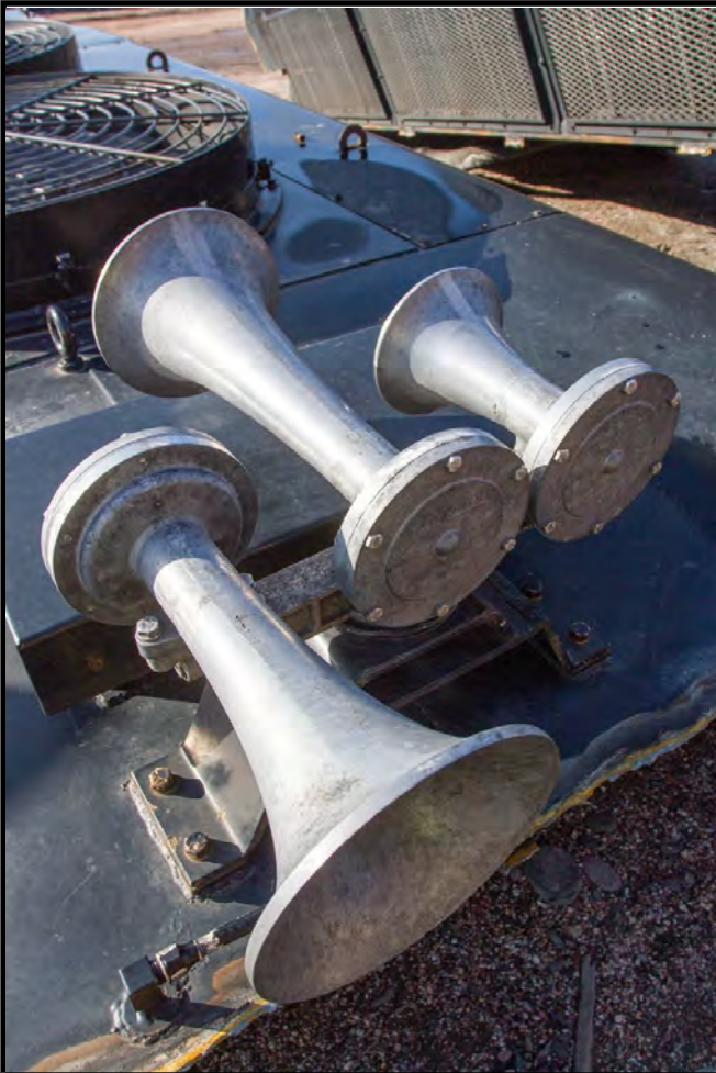
Three-chime Nathan Airchime air horns are still common, but most new locomotives are equipped with five-chime
