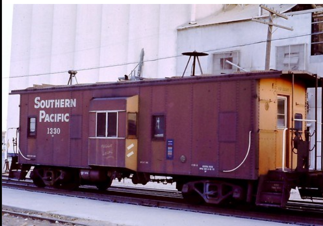
Bay-window Caboose (photo from trains.com)
