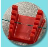
designed to hold two wires securely while one solder-spliced the wires together:
