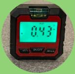
also brought in a digital level that shows degrees of change. He uses both tools to help determine the grade for his track when creating climbs and descents.
