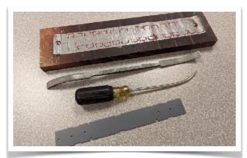
Some of Mark's "custom made" tools: a block of wood with duct tape thumbtacked in place, to temporarily hold seats and detail parts for painting; a curved file for smoothing out the car shell's floor; a bent screwdriver which Mark uses to help pry up hard to reach components; and on the bottom, a machined steel floor weight (Mark offers a variety of these steel weights – check his website).
