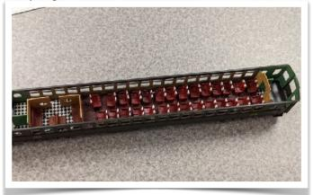
A view of the complete interior installed. Note the "tile" floor to the left in the smoker's compartment.
