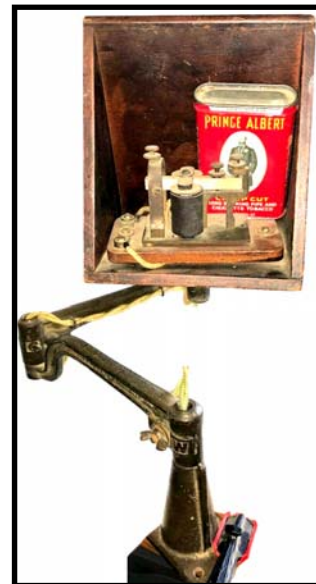
Figure 9. Western Electric Telegraph Sounder Mounted in Resonator
