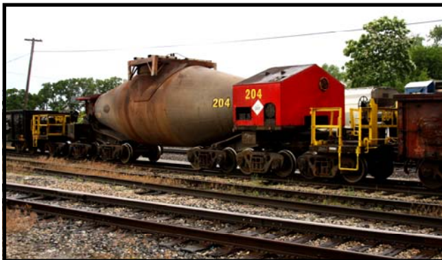
A very uncommon sight around here is this bottle car used in steel mills.
