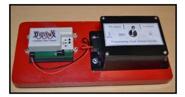
PR4 Programming Interface and Programming Track Selector Switch
