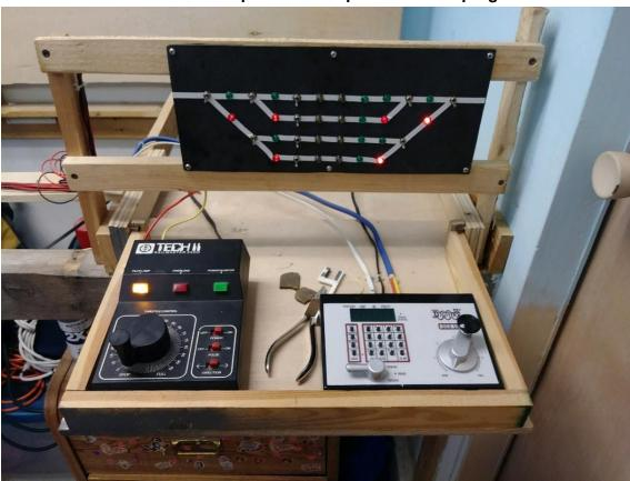
Control Panel for 4 track staging. 6 Tortoise machines and all the lights and switches was close to 100 solder connections.
