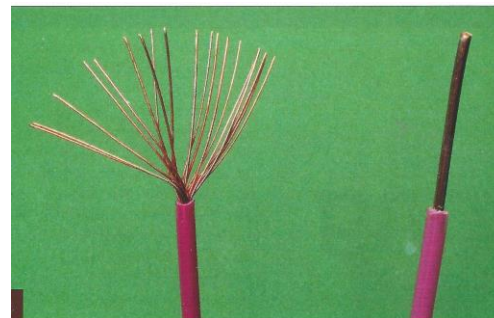
Wire is either stranded (left) or solid. Stranded wire is more flexible than solid.
