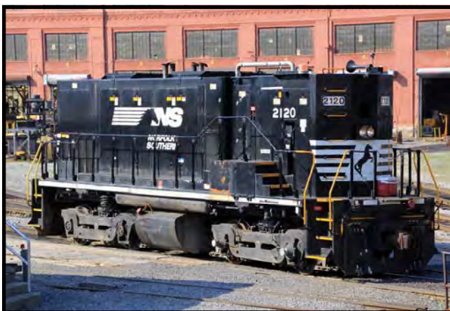
NS #2120 is a cabless genset unit rebuilt with Rail Power Technologies power units at NS TMS Altoona shop in 2008 on an SW1500 frame.
