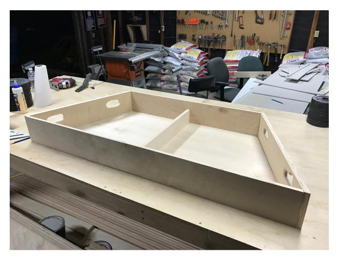
In **Figure 2**, the first completed frame is shown. When this was assembled, a little miscommunication occurred, where a previously cut end plate was used and then cut again to line up with the side frames. That left the plate a little on the short side. The hand holes were cut freehand with a router, which slipped during the process.
