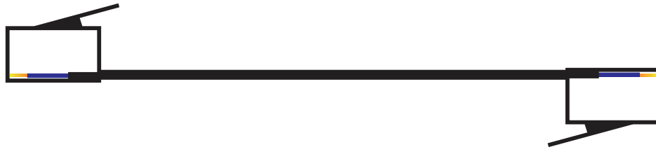
Figure 4. Straight through LocoNet cable ó Note that the blue outside wire is in the same location relative to the tab on each connector plug. (Schematic by Frank Wilhelm)
