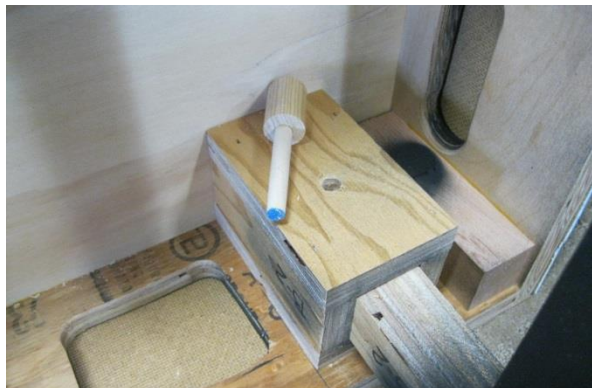
Figure 3. Leg pocket with key-hole lock. Also, note corner brace. (Alan Ashton photo)
