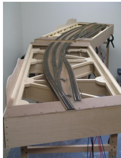
Figure 2. Diagonal bracing and solid top surface at the endplate add considerable strength to longer modules. (Frank Wilhelm photo)
